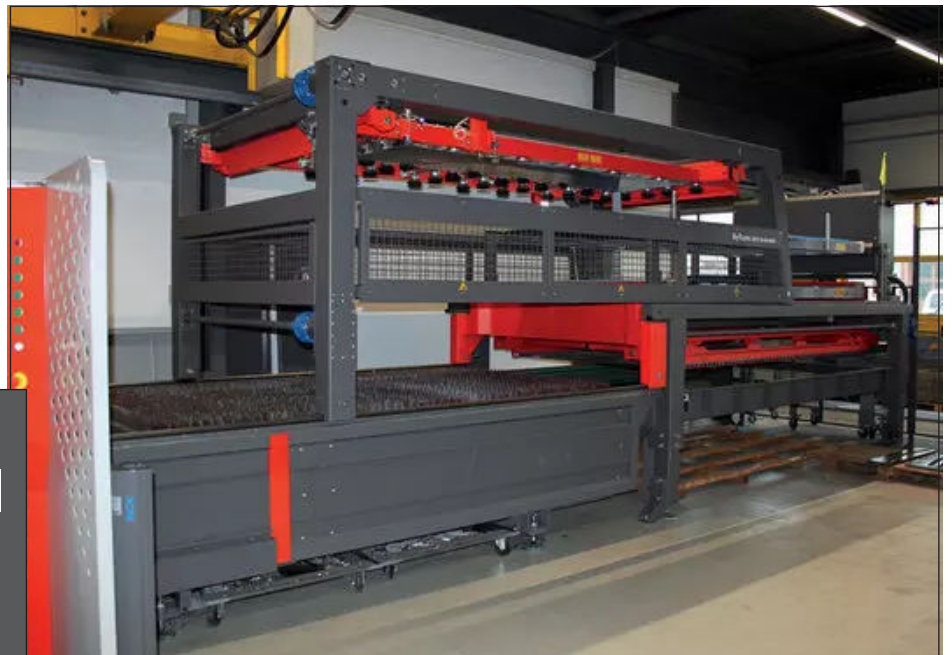
Above and below: The ByTrans automatic loading and unloading system on the new laser cutting machine for self-sufficient, fully automatic order production in all batch sizes. On the right is the pallet loading/unloading station.
