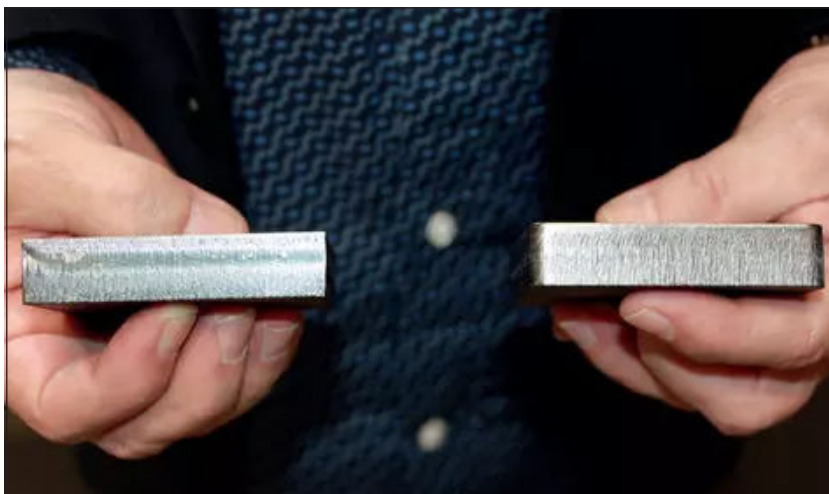
The direct comparison of power laser cutting without gas (left) and with gas (right). Depending upon the material and cutting speed, deburring and/or surface grinding operations are also unnecessary.
